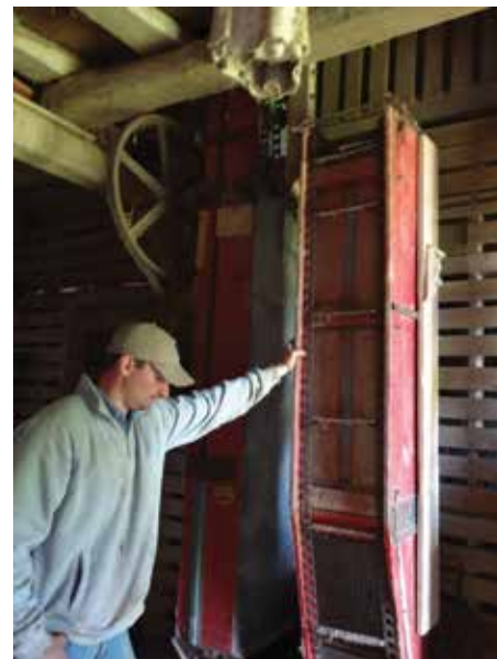
Figure 4: The grain hopper in the alley was either below ground level or lowered to the floor level after the corn wagon was in position. Aarik Deering. PHOTOGRAPHED BY MARLENE FENSTERMANN MAY 15, 2016.
