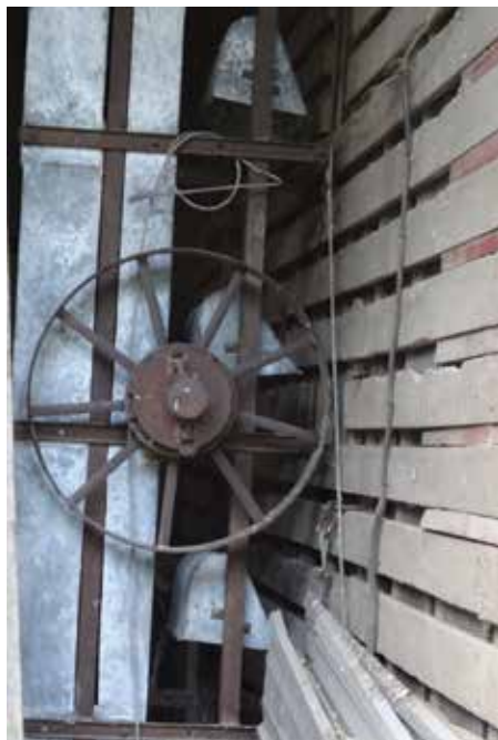
Figure 3: Vertical elevator metal shaft on the left. Metal buckets on the right traveling downward to the floor hopper to be filled with grain. Photo detail from the corn crib shown in Figure 2.
